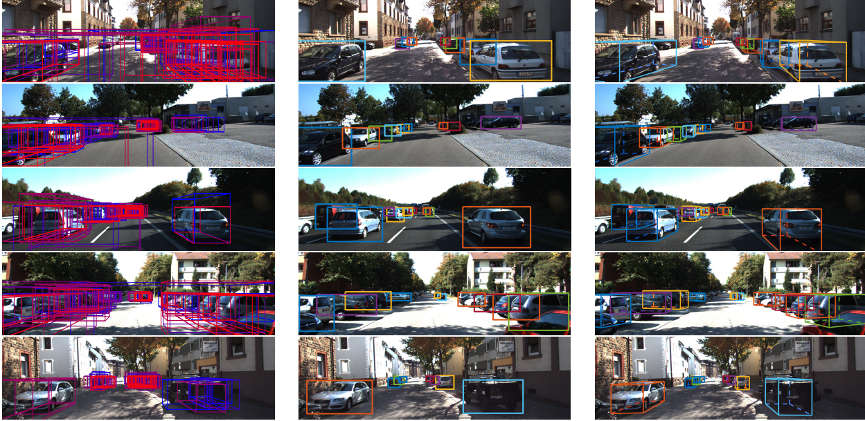
Figure 7: Qualitative examples of car detections results: (left) top 50 scoring proposals (color from blue to red indicates increasing score), (middle) 2D detections, (right) 3D detections.
